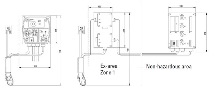
Figure 2 Sample probe type ASP 611 controller Figure 3 Sample probe type ASP 613 controller
