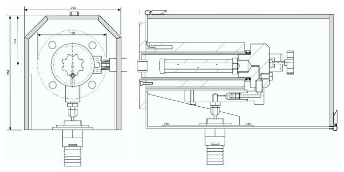
Figure 1 Sample probe type ASP 61x drawing
